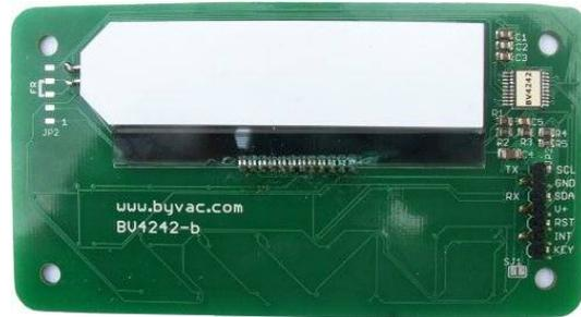
The interface is very simple with a 7 pin connector designated as follows:
